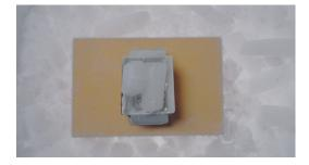
h. After **5 min**, remove mold B and determine if the OCT is completely frozen and has turned opaque. If it is not completely frozen and opaque, repeat step f.
